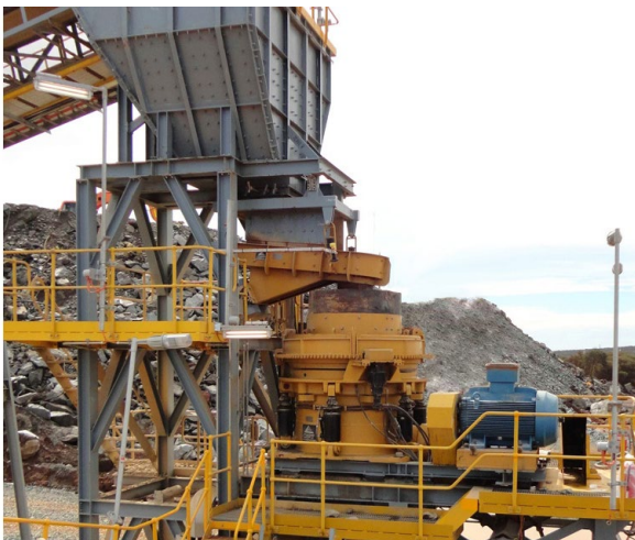
Trio® cone crusher operating at a zinc, copper, gold mine facility in Western Australia.
